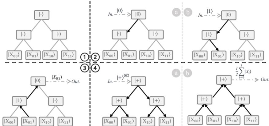
Figure 2: A bucket brigade QRAM. Note that, in this picture,  $|wait\rangle = |\cdot\rangle$ ,  $|left\rangle = |0\rangle$  and  $|right\rangle = |1\rangle$ . In **2** and **3**, we access the address 01 of the memory, and the change of the qutrits is shown. In **4**, an access in superposition is shown (two  $|+\rangle$  states are the input), and we get as output an equiprobable state of the contents of addresses 00, 01, 10 and 11. Taken from [16].
