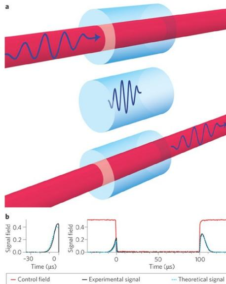
Figure 3: Image of an Electromagnetically Induced Transparency quantum memory. The state to store, codified in the blue photon beam, can pass through the medium while the control signal (red laser) is active. Figure taken from [12]
