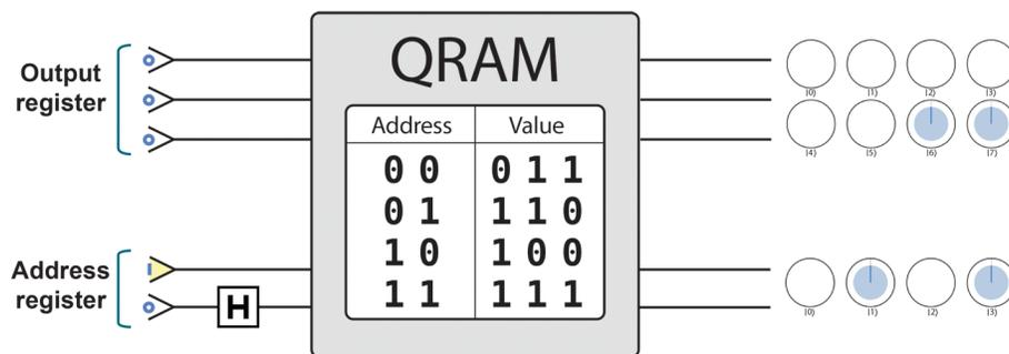
Figure 1: Example of an abstract quantum memory that stores classical information. In this case, the memory is accessed in an equal superposition of the states  $|01\rangle$  and  $|11\rangle$  created by applying a Hadamard gate to the most significant bit, thus obtaining an also equal superposition of the values stored at those addresses:  $|110\rangle$  and  $|111\rangle$ . From the book *Programming Quantum Computers* [10].
