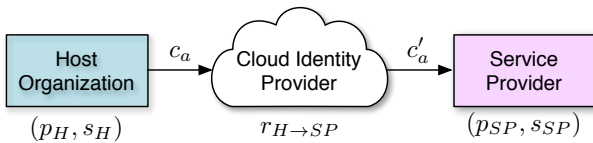
Fig. 6 Data flow of BlindIdM
