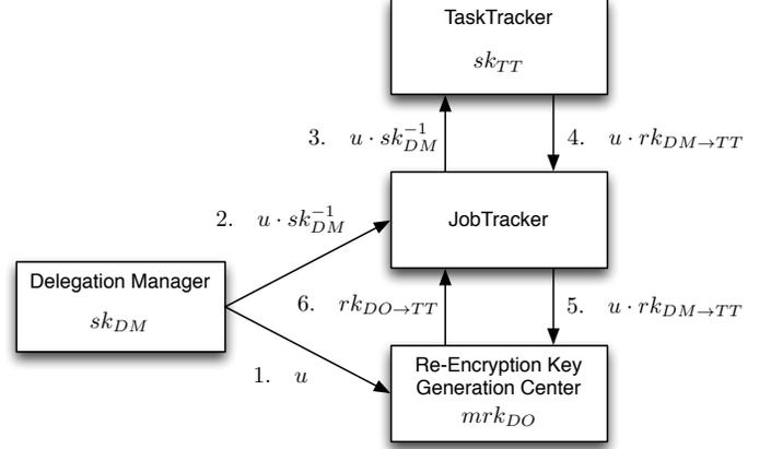
Fig. 2. Re-Encryption Key Generation protocol
