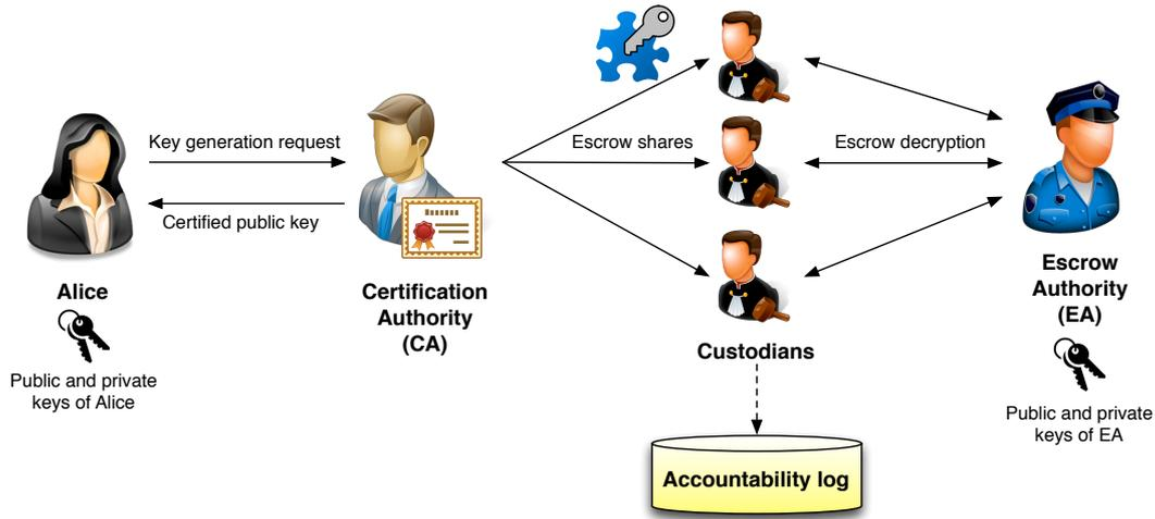
Figure 1: High-level view of actors and interactions in an escrowed decryption system
