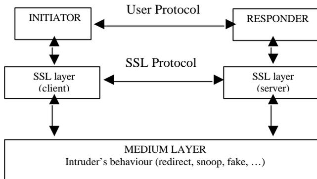
**Figure 2: Modules Schema of security system specification**
