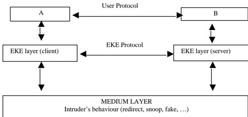
**Figure 4: Multilayer structure of EKE environment**
