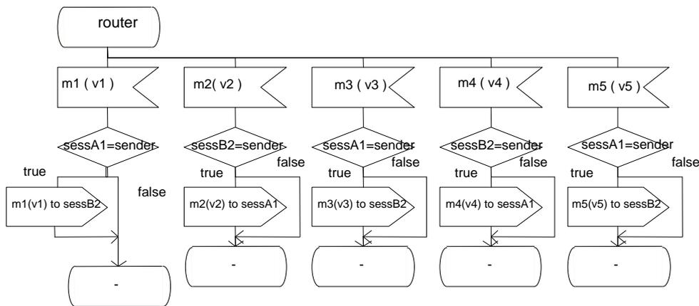
Figure 6: Main state of "CorresAttack" process
