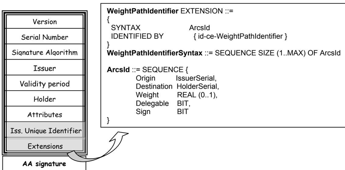
**Figure 1: Attribute certificate and weight path identifier extension.**
