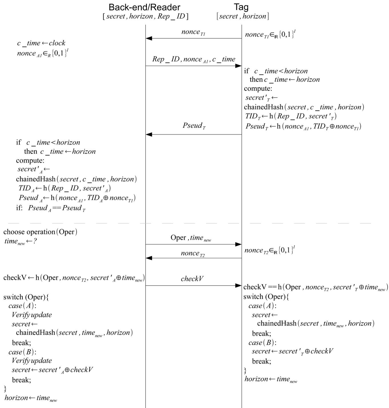
Fig. 1. Compact schematic of Tag Query
